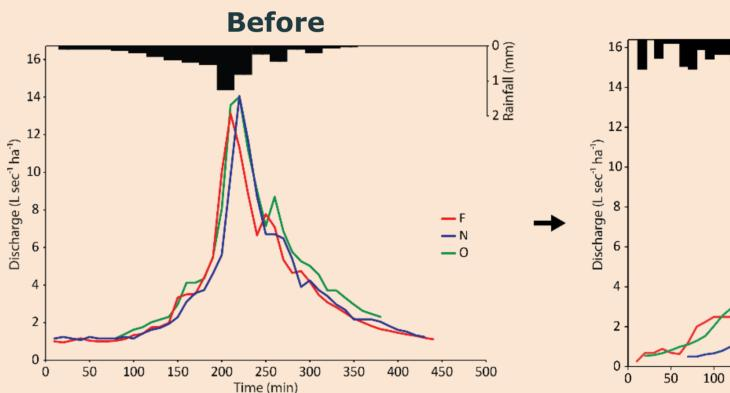
Hydrographs produced in bare peat catchments flashy, are characterised by short lag times and high peak discharges.
