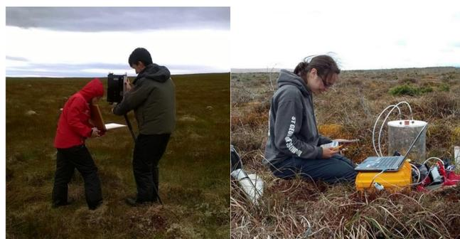
To test the model at a small scale in the field we used a handheld spectroradiometer and a flux chamber to measure surface reflectance and carbon fluxes across the growing season.
