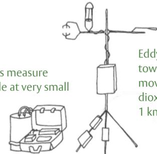
Eddy Covariance (EC) towers measure the movement of carbon dioxide at scales of 200 m to 1 km.
