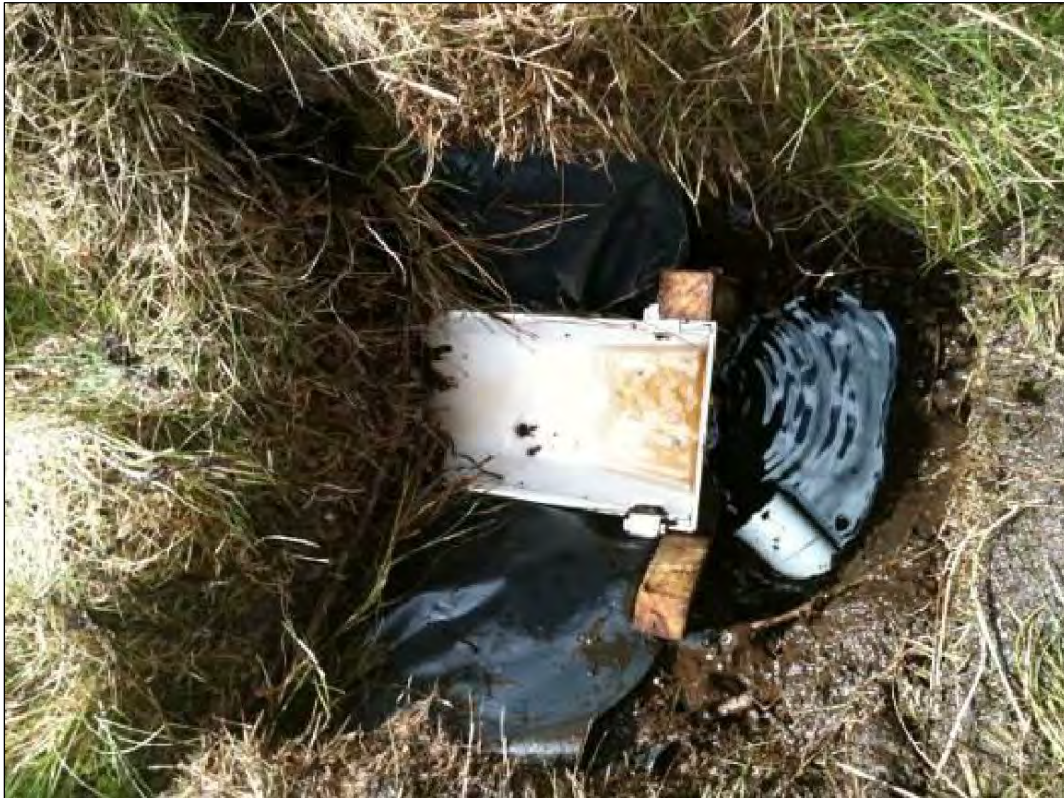
Photo E1: Furrow chamber located at the bottom of sub-block, downhill of the vegetated buffer left in place as a deliberate part of the block design (this mimics the real operation, where buffers are left in place). Chambers were installed by exposing the base of an old plough furrow, creating drainage out to the downhill side and then creating a place (plastic gutter) where runoff samples could be obtained for water quality testing (furrows were judged to be the main flow paths off the trial sites, and obtaining samples in drought conditions would be difficult if not located in these places).
