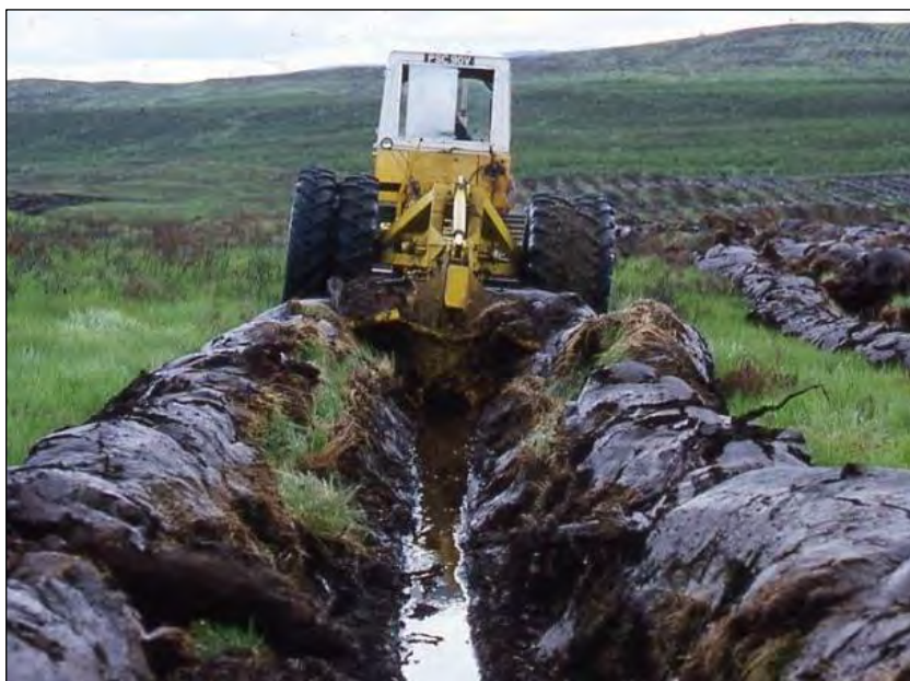
Photo 1: Forestry ploughing on peatland (courtesy of http://www.forestry-memories.org.uk/ ). This image shows a double mould-board plough which throws a turf ridge up on either side of the furrow. Other ploughs (single mould-board) throw only one turf ridge up per furrow.
