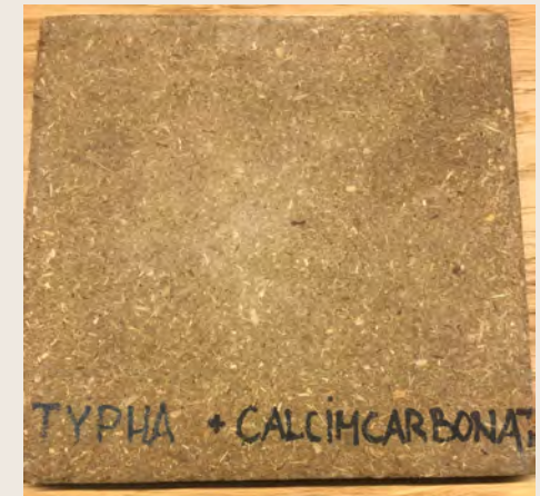
Typha & Calcium Carbonate - creates a stronger cementitious-like board
