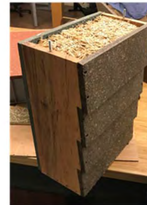
(left) inspecting seed heads of Typha latifolia and (right) fibre board and insulation from this crop – Jim Milner
