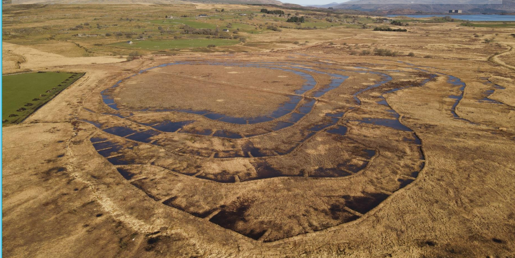
Contour bunding installed at Cors Goch Trawsfynydd SAC winter 2022/23 – taken from a drone.
