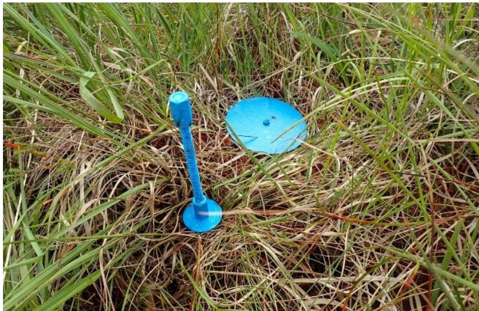
Example of an installed rust-rod & surface-level marker
