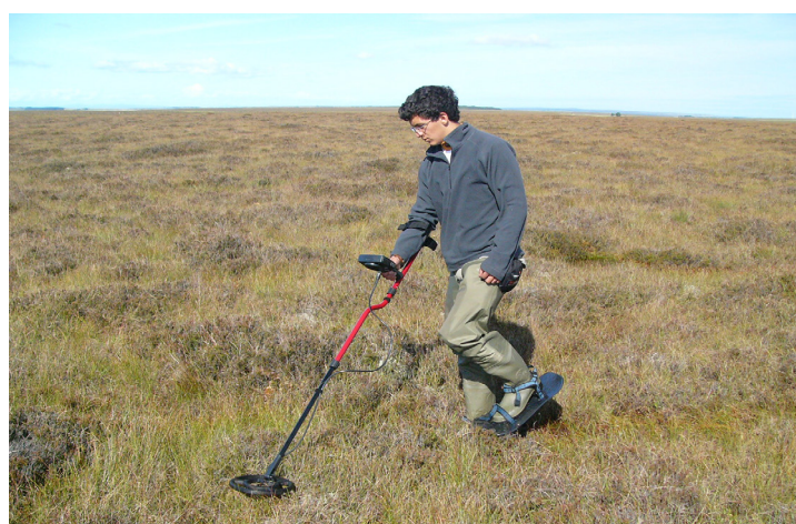
Locating surface-level rods with a metal detector.
