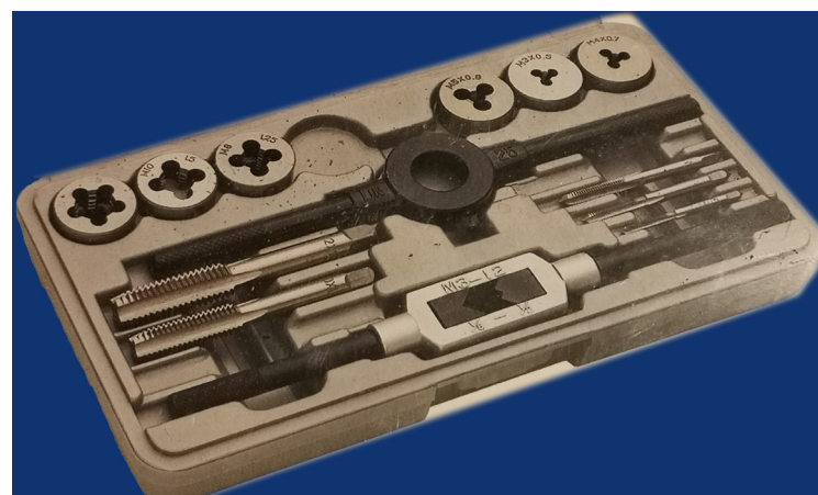
Threading die kit which can be used to add threads to the top of mild steel rods for attaching the washer assembly.
