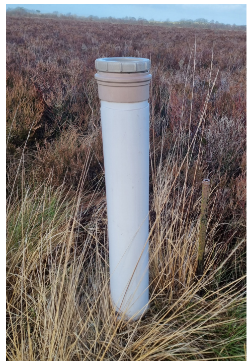
Dipwells consist of a plastic pipe set into the peat.
