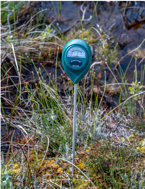
Moisture meter used to determine surface-pattern zone or ‘tope’ according to the depth at which high moisture is reached (blue colour on the dial).
