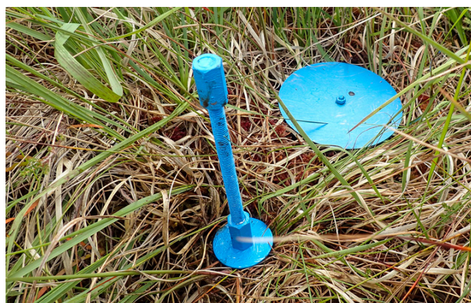
Surface-level rod (left) with adjacent rust rod (right)
