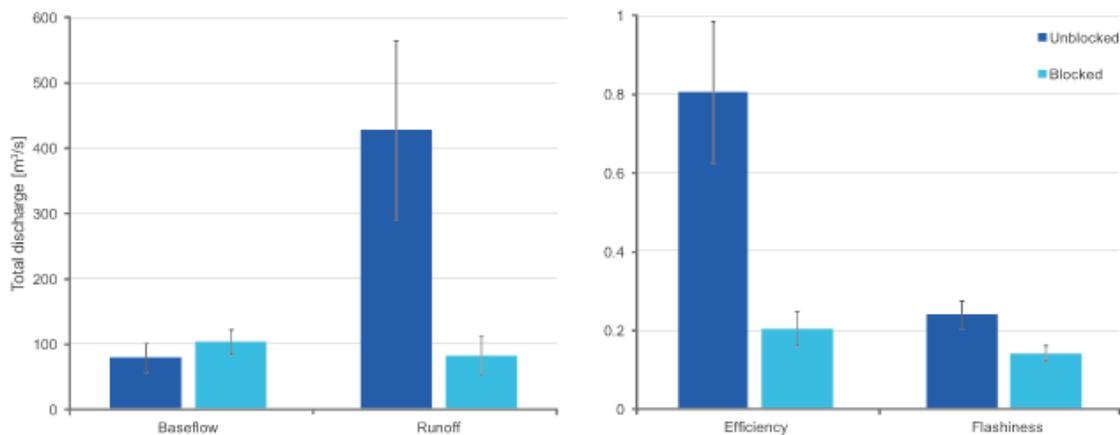
**Figure 11** Change in baseflow and runoff after grip blocking. Blocking grips leads to reduced runoff with more water retained on the bog (Efficiency index) and a less concentrated flood response (Flashiness index). Data from Lorraine Wilson, see also Wilson et al. (2010; 2011a)
