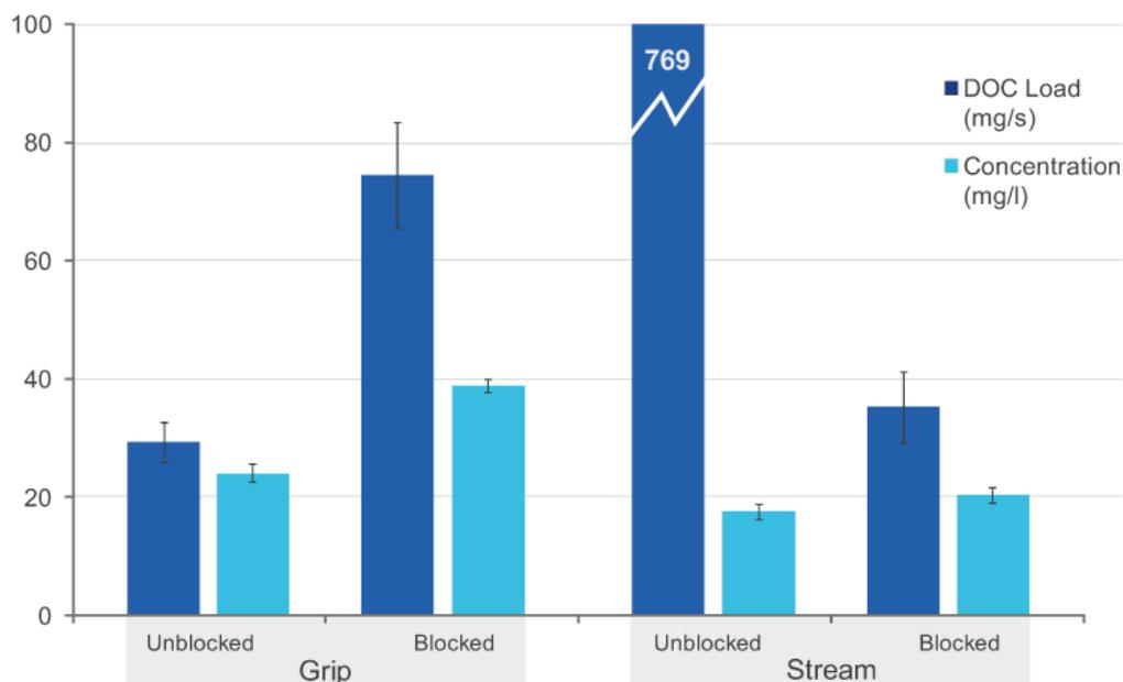
**Figure 10** Effects of grip blocking on DOC levels. While DOC levels initially increased in grips after blocking in the first 18 months, overall DOC concentrations in streams, however, did not change and reductions in flow led to very large reductions in load (data from Lorraine Wilson, see also Wilson et al. 2011b)
