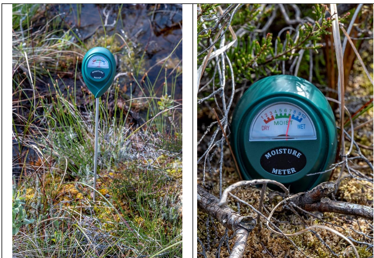
Figure 5. Examples of simple 30 cm moisture probes indicating differing depths of the high-moisture zone and thus presence of differing nanotope zones.
