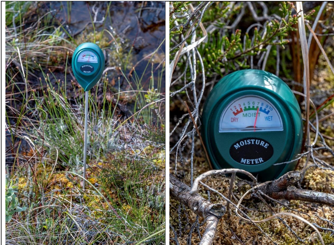
Figure 3. Use of a simple 30 cm soil moisture probe to determine the depth at which the zone of exceptionally high-moisture zone is located within the peat, thereby indicating the synusial zone. In this case (left) a T1 low ridge, and (right) a T3 hummock).
