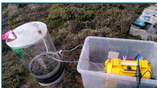
Fig 2. A field Infra Red Gas Analyser.
