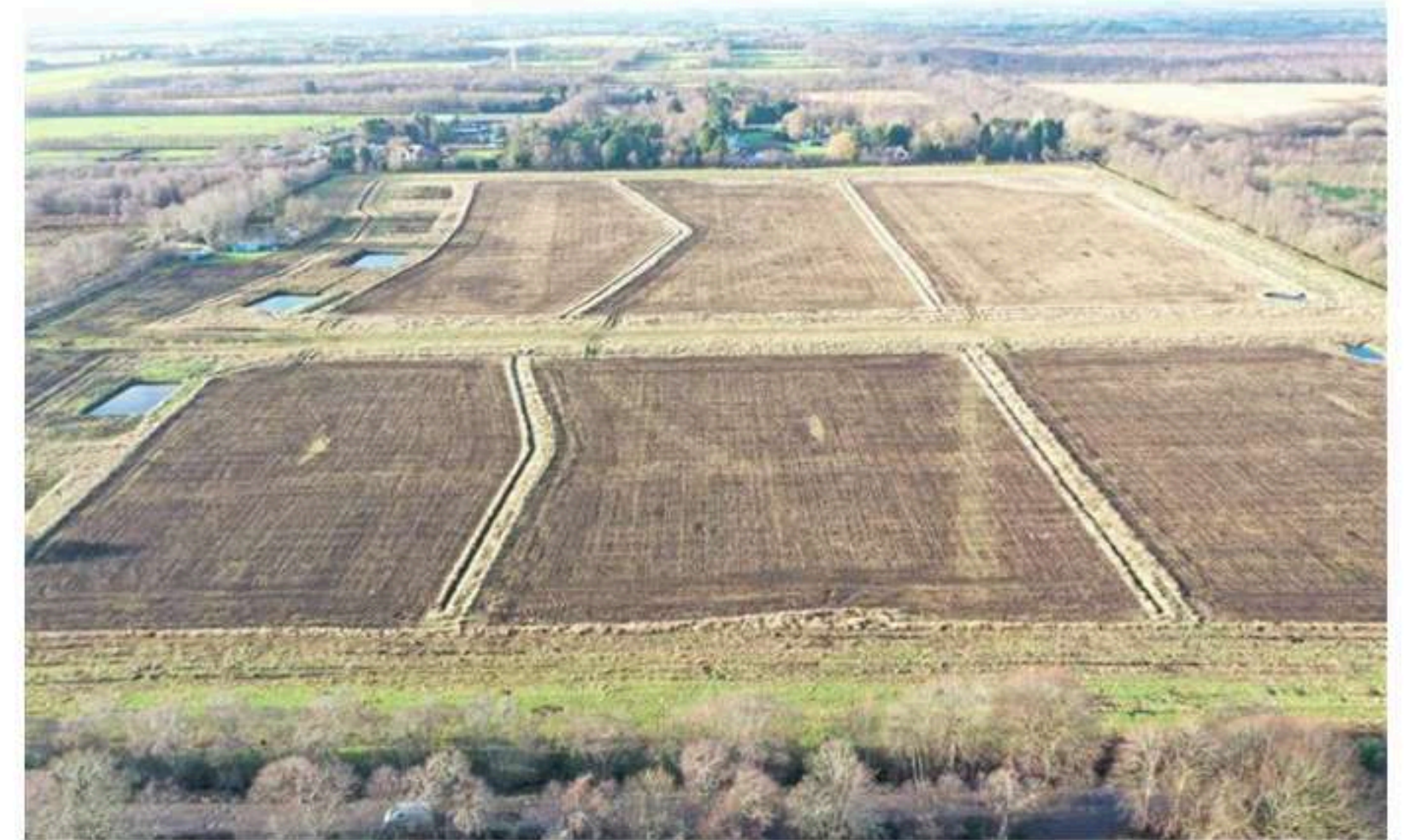
Capital works including deep trench bunding, cut-off ditches, water retention ponds and sluice gates to control in-field water levels
