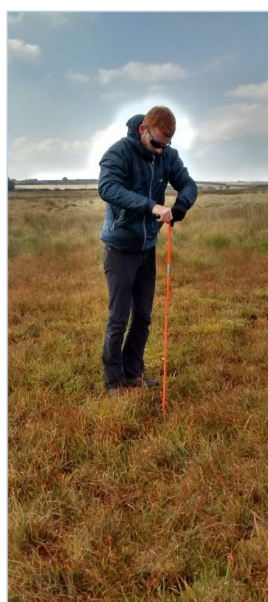
Fig. 2 Gathering peat depth measurements in Exmoor National Park, October 2015.
