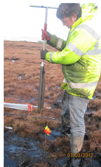
Figure 60 A Russian corer provides a half cylinder of peat. Compaction is minimal and the sampler is easy to use © Julia McCarroll
