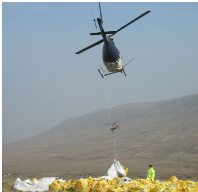
Figure 134 Helicopter lifting bags of heather brash for use in bare peat restoration © Yorkshire Peat Partnership
