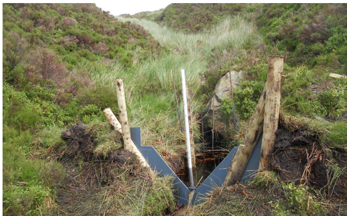
Figure 54 A v-notch weir with a dipwell and a turbidity flow meter installed in the North York Moors.
