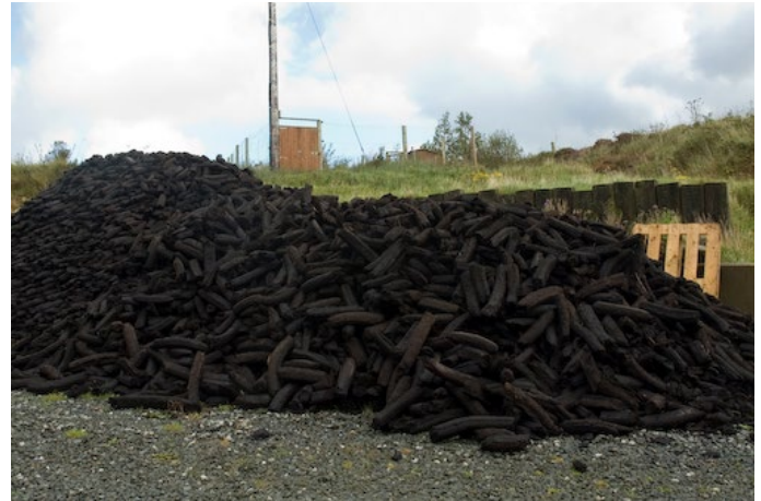
Figure 25 Mechanised sausage cutting. Sites cut in this fashion are particularly difficult to manage as much of the active drainage is sub-surface. This method of cutting is replacing more traditional techniques, particularly in the Scottish Highlands and Ireland © Steve Wilson
