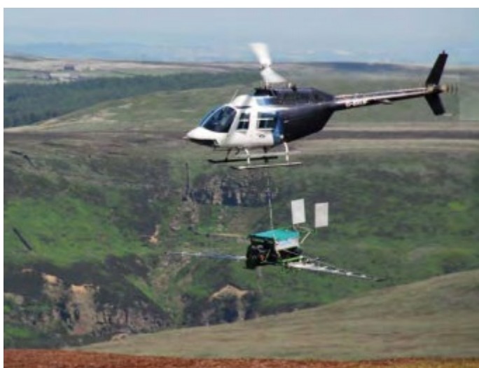
Figure 140 Helicopter application of grass seed © Moors for the Future Partnership
