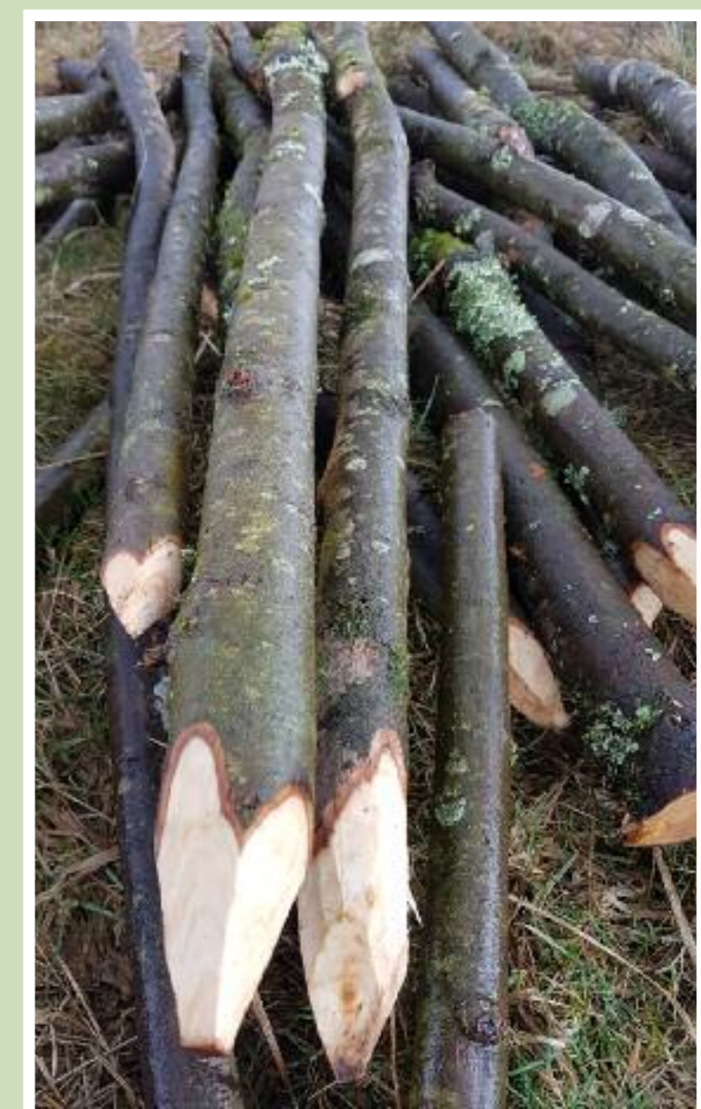
Right: Locally sourced grey willow was used. Cut and constructed by Heart Wealden Enterprise Ltd. Dimensions of the fascines 2500mm x 400mm., and stakes 1500mm.
